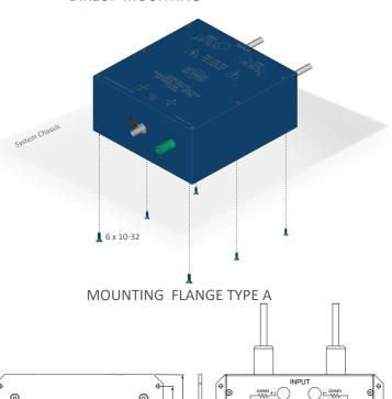
DP40 series probes can be mounted directly on a base plate or enclosure walls with 6 x 10-32 screws.
